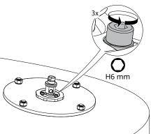
2. Rotate the antenna so the air purge connection is directed toward the tank wall.
