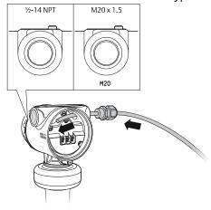
5. Connect the cable wires.
