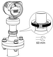
7. Carefully lift the transmitter head.
