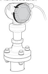
5. Remove all electrical leads and disconnect conduit.
