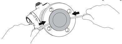
2. Gently push the screwdriver handles forward until the PTFE sealing pops out.
