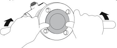
3. Carefully pull the PTFE sealing straight out.
