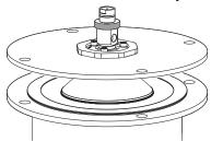
10. Tighten the bolts and nuts with sufficient torque for the flange and gasket choice.
