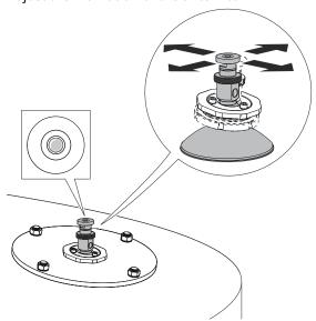
5. Gradually tighten the M8 screws.
