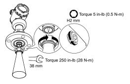
5. Place a suitable gasket on the tank flange.
