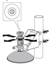
5. Gradually tighten the two M8 screws.
