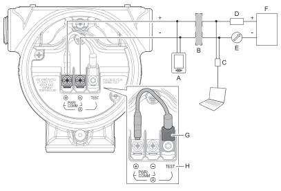
Figure 4-5: 4-20 mA/HART Communication - Terminal Block with TEST Terminal
