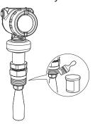
5. Lower transmitter with antenna into the nozzle.
