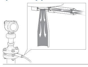
Flushing connection rings are available as accessory for use with process seal antennas.
