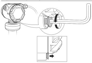
d) Turn the jam screw an additional ½ turn counterclockwise to secure the cover.
