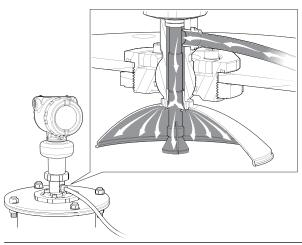
An air purge connection is also available for cone antennas with flanged connection by selecting option code PC1. This option consists of an antenna with purge holes and a separate air purge ring (see Figure A-11).
