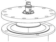
3. Tighten the bolts and nuts with sufficient torque for the flange and gasket choice.
