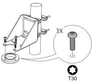
3. Unscrew and remove the antenna.
