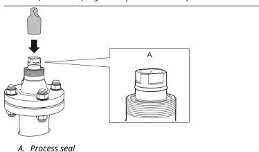
8. Attach a protection plug to the process seal to protect it from dust and water.
