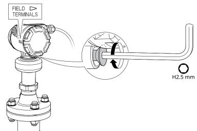
3. Turn the jam screw clockwise until it is completely threaded into the housing.
