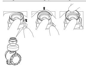
2. Replace the transmitter head nut.
